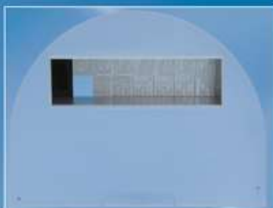
40 mm basic test phantom with aluminium step wedge
